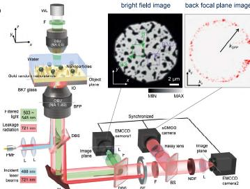
Validation measurements: bright field and fluorescence microscopy used to independently verify particle binding.
