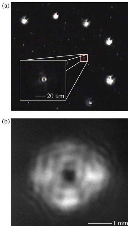
Fig. 2. (a) Curved path described by the fiber bundle at the exit side. The white box is a magnified image of the overlapped orders when creating a partially coherent doughnut beam. The partially coherent doughnut beam is produced by incoherently superposing HG mode (1, 0), mode (0, 1), and mode (1, 1). (b) Irradiance distribution of the partially coherent doughnut beam at the back focal plane of the collimator lens.
