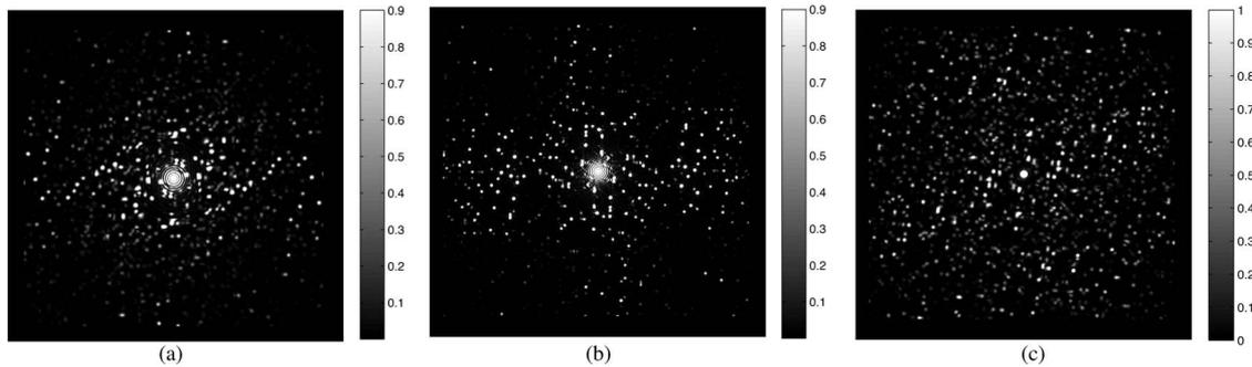
Fig. 3. (a) Fourier spectrum obtained experimentally when illuminating the pinhole array with the generated partially coherent doughnut beam. (b) Theoretical Fourier spectrum expected when illuminating the array with the generated doughnut beam. (c) Experimental Fourier spectrum obtained when illuminating with a fully coherent doughnut beam.
