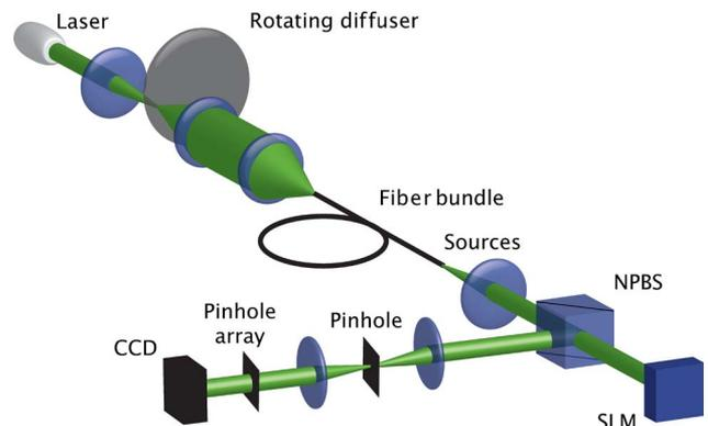
Fig. 1. (Color online) Schematic of the experimental setup proposed for the generation and characterization of structured partially coherent beams. NPBS, nonpolarizing beam splitter.
